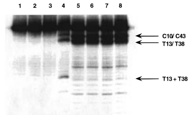
**Figure 7.** Cleavage of hairpin oligonucleotide by **6** activated with Fe(II)-O<sub>2</sub>. Lane 1, hairpin only; lane 2, hairpin + Fe(II); lane 3, hairpin + **6**, no Fe(II); lane 4, 20  $\mu$ M bleomycin A<sub>2</sub>; lane 5, 10 s digestion with 300  $\mu$ M **6**; lane 6, 30 s digestion with 300  $\mu$ M **6**; lane 7, 60 s digestion with 300  $\mu$ M **6**; lane 8, 120 s digestion with 300  $\mu$ M **6**.
