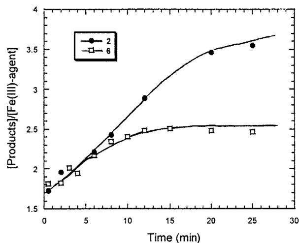
**Figure 8.** Kinetics of styrene (50 mM, 30 mM H<sub>2</sub>O<sub>2</sub>) oxidation catalyzed by the Fe(III) complex of agent **2** and **6** (500  $\mu$ M). The ratio of total concentration of products (styrene epoxide and phenylacetaldehyde) versus the initial concentration of Fe(III)-agent complex (turnover) is plotted against time.
